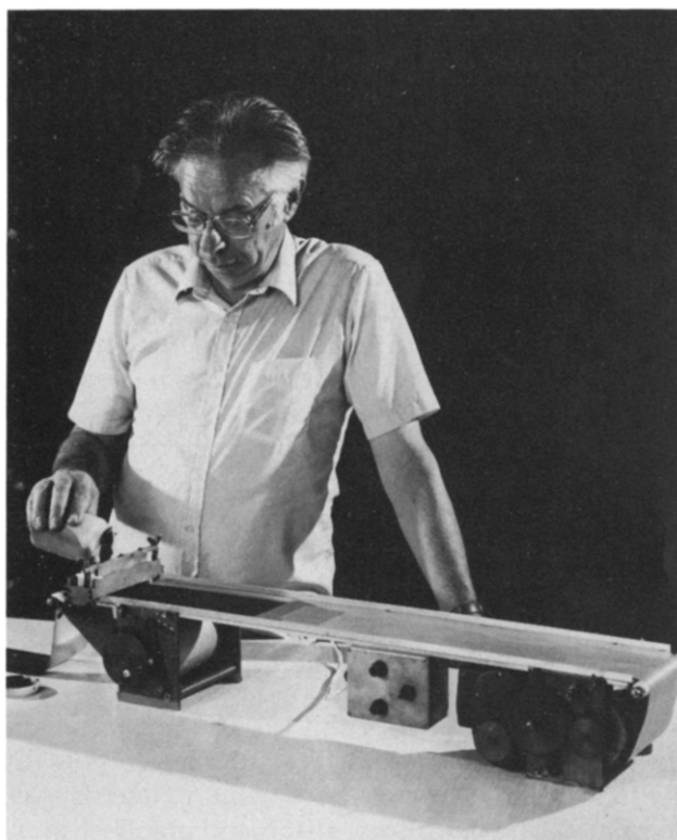
Fig. 1. The fabrication of an all-solid-state composite cathode using a continuous-casting, solvent-evaporation technique.
